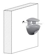
Recommended fixing countersunk screw type - head  $\varnothing$  5 mm max.
