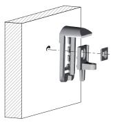
Recommended fixing countersunk screw type - head  $\varnothing$  5 mm max.
