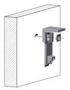
Recommended fixing countersunk screw type - head  $\varnothing$  5 mm max.
