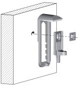
Recommended fixing countersunk screw type - head  $\emptyset$  5 mm max.
