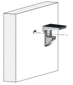
Recommended fixing countersunk screw type - head Ø 5 mm max.
